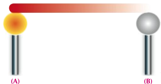
▲ Figure (5) : Heat transference by conduction
