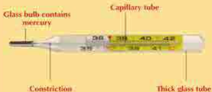
Fig (2-6): Structure of medical thermometer
