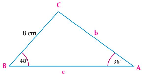
$$\therefore \frac{a}{\sin A} = \frac{c}{\sin C} \quad \therefore \frac{8}{\sin 36^\circ} = \frac{c}{\sin 96^\circ}$$
