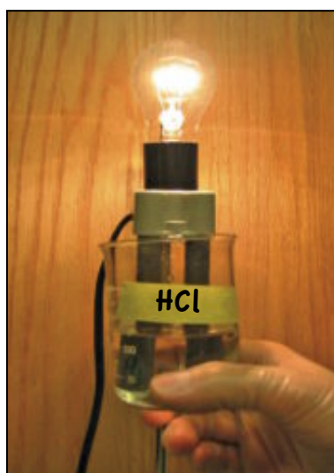
▲ Figure (13) A strong acid conducts an electrical current to a greater extent than a weak acid
