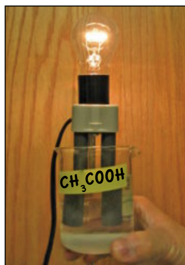
▲ Figure (13) A strong acid conducts an electrical current to a greater extent than a weak acid
