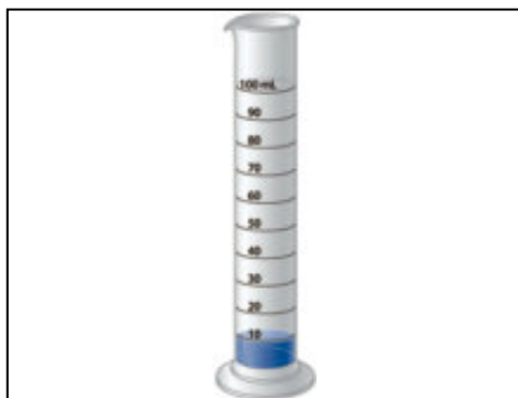
▲ Figure (7) Used to determine the volume of a liquid in a cylinder
